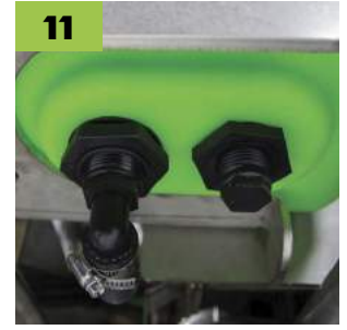
Tank Sump with Drain
